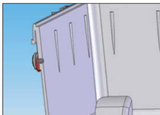
Inside wall thickness removed behind purge valve area to increase internal volume
