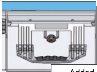
Added overmolded front and side handles
